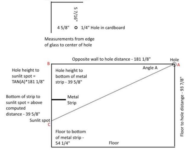
First of all here is some info. The right side of the diagram represents the wall with the window. The left side is the wall with the strip of paper. The top is a level line from the hole at the window to the wall opposite.
